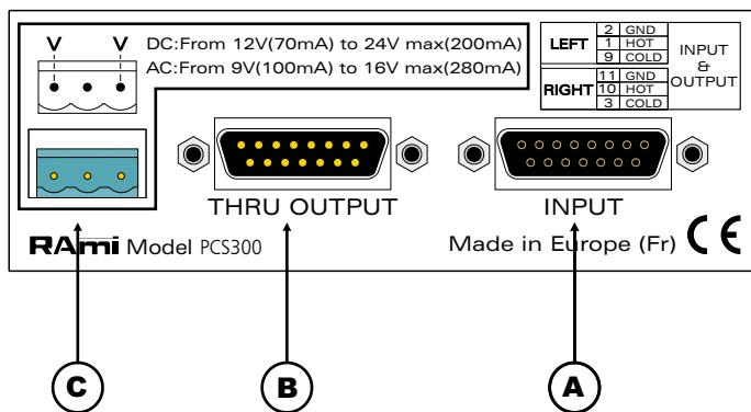
**A -** Balanced stereo analog signal input.
