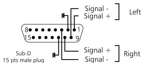
**B -** "THRU" output (analog). Outputs the signal from (1) to interconnect several PCS 300.
